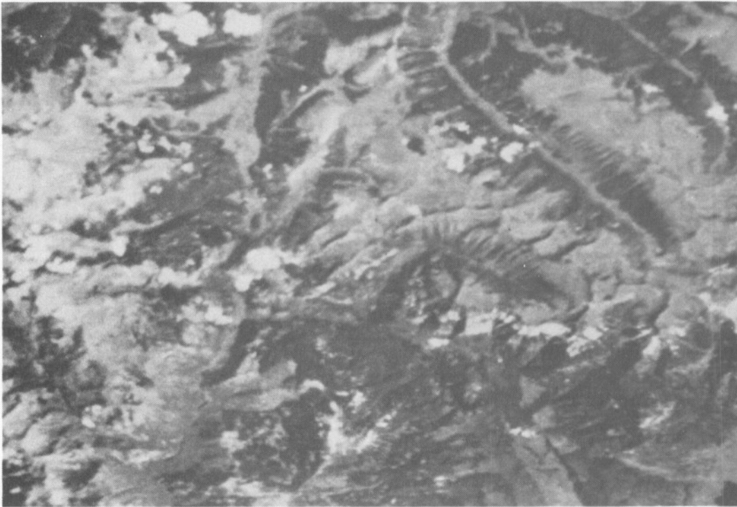
Figure 7. Enhanced color infrared composite of ERTS-1 imagery from the LARS digital display unit, showing avalanche track locations. The scale of this illustration is approximately 1:150,000. This data was obtained on September 8, 1972. Similar enlargements have allowed forest clear-cuts and burned areas to be delineated. Such computer-aided enhancement and enlargement capabilities offer many advantages for effective utilization of ERTS data in various application areas.
