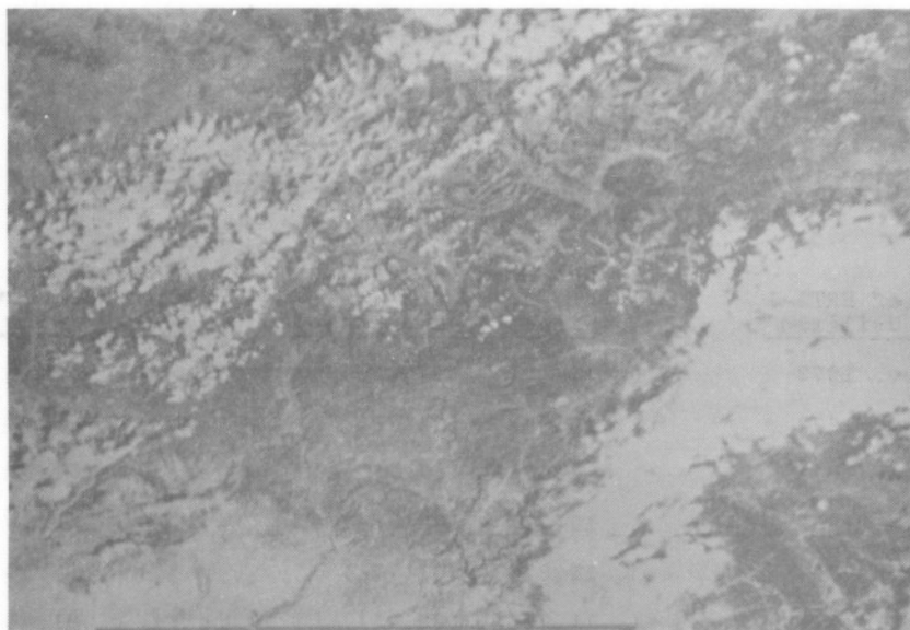
Figure 1. Color-infrared composite of September 8, 1972 ERTS-1 data from the San Juan Test Site in southwestern Colorado, taken from the LARS Digital Display Unit. The scale lines indicate a 100 kilometer (62 statute miles) length. Two different scale lines are necessary because rectangular ERTS-1 data elements are being displayed as square picture elements on the digital display.
