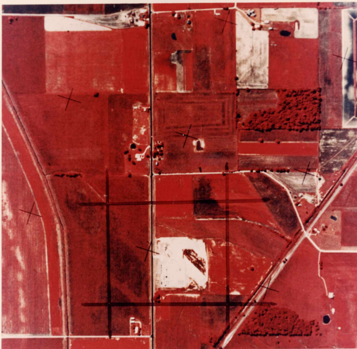
Figure 1. Digital Display Photograph of the .59-.71 micron (Red) spectral channel of the agricultural test site used in the study.
