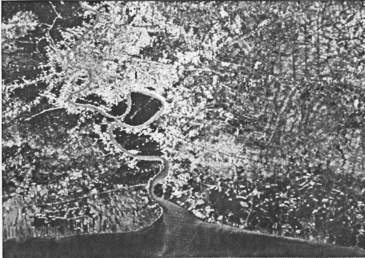
Figure 4. False color image of Bangkok, Thailand study area, produced from Landsat MSS bands 4, 5 and 7.
