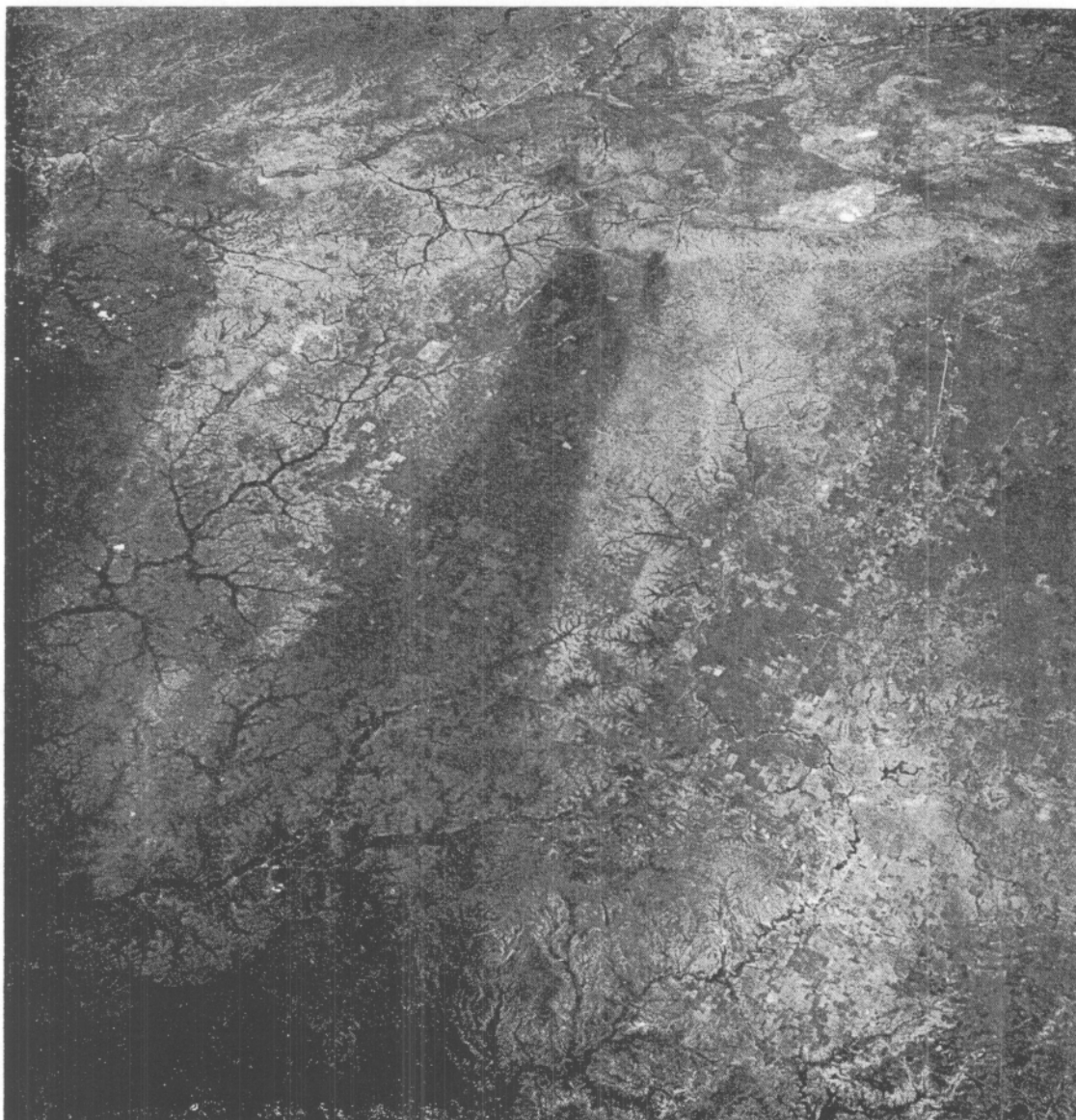
Figure 31. Rain patterns in Texas, as photographed from Gemini IV at an altitude of 102 miles. The dark-toned areas correspond to the path of a rain storm the previous day.
