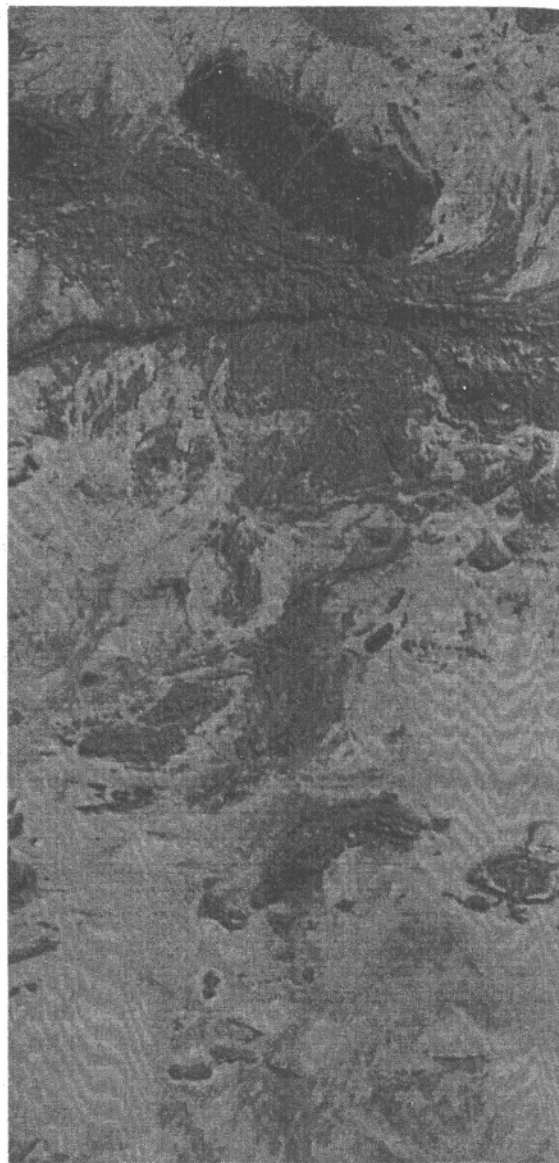
Fig. 10. Colour composite from CCT displays of bands 4, and 6, and the ratio image of bands 5/7 printed as blue, green and red respectively. Scale approximately 1:500 000
