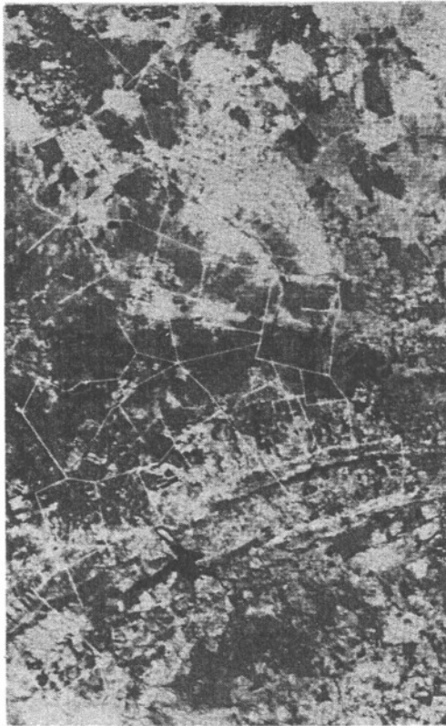
Fig. 1. Part of CCT-1 of frame No. 1049-07301 showing composited cadastral features as white lines. Scale approximately 1:500 000.
