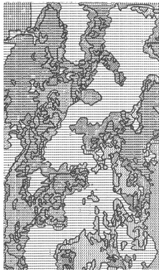
Figure 2. Computer Soil Classification Map of Test Site. Legend: (M) Ragsdale silty clay loam, (F) Brookston silty clay loam, (O) Toronto silt loam, (C) Celina silt loam, (-) Reeseville silt loam, (/) Crosby silty loam, (I) Brookston silty loam, (A) vegetation.
