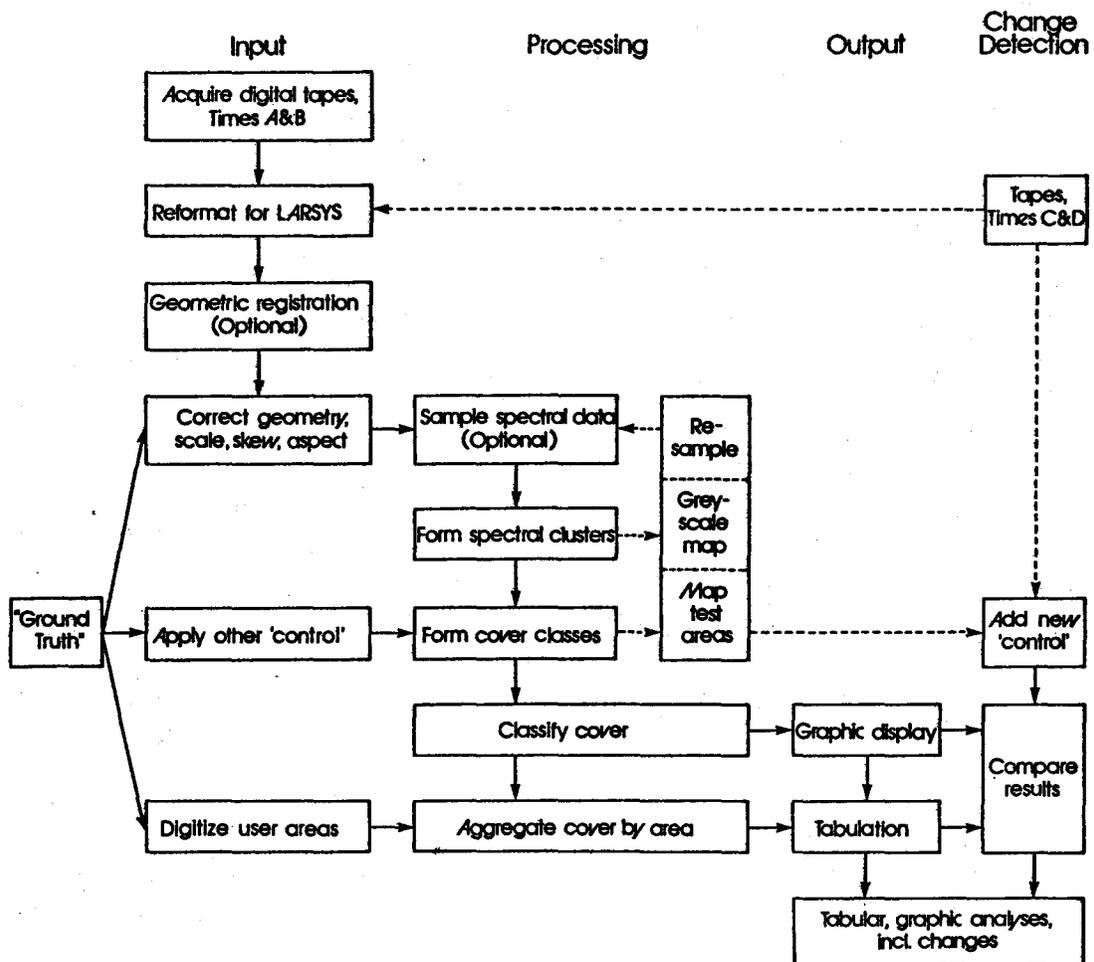
Figure 1. Procedures for Computer-Aided Classification of Land Cover from LANDSAT Multispectral Scanner Data<sup>1</sup>
