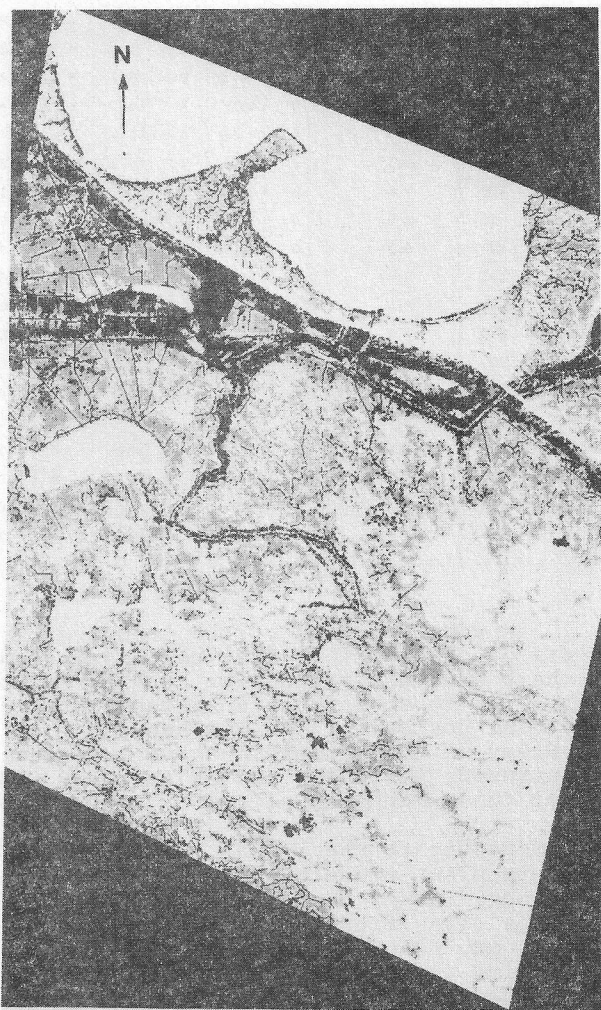
Figure 9. Classification of Productive Capacity for the La. Marsh Test Site. The PC values are relative and dependent on plant production, water body type, and distance to nearest water for each Landsat cell identified as marsh. Areas of high PC are light gray, medium PC are medium gray, and low PC are dark gray. Water is white and non-marsh is black.
