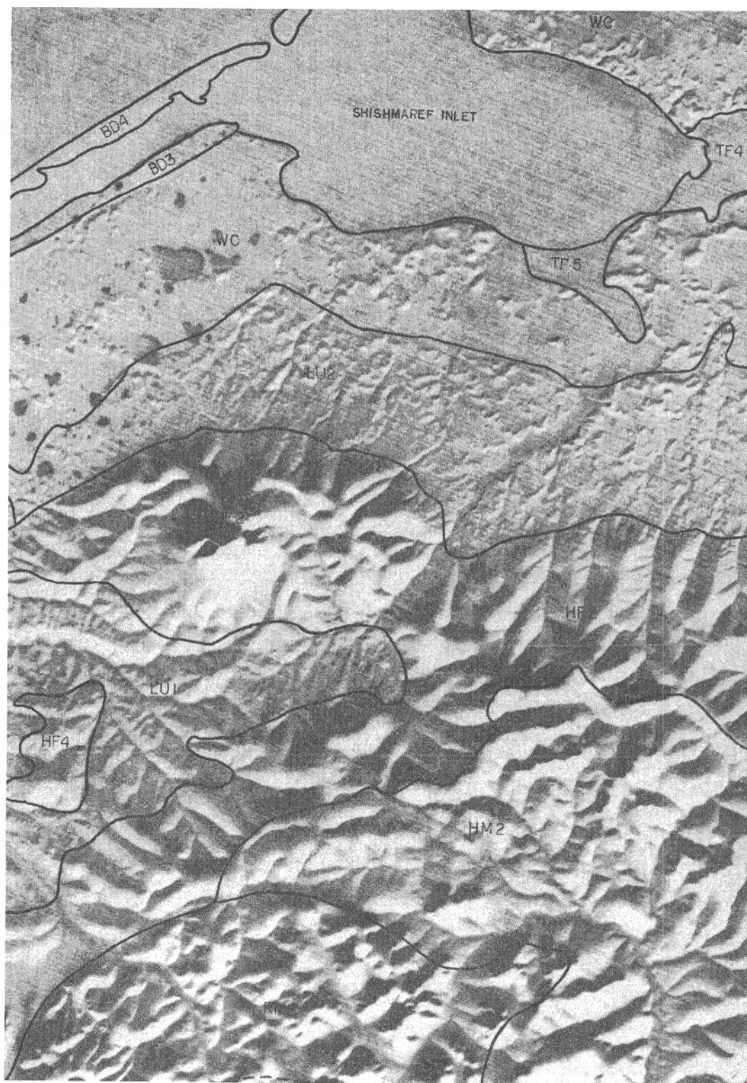
FIGURE 4. Physiographic Units. The units are shown here on the winter Landsat image from which they were interpreted. Table 1 is the key for these units. Figure 2 shows the physiographic unit map derived for the entire project area.
