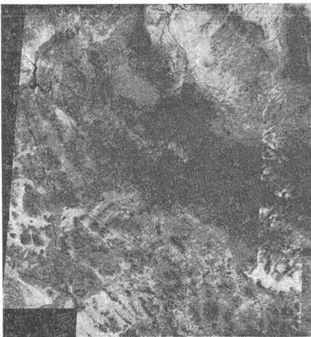
Figure 1: Arizona State Mosaic . This image is 10,300 lines by 9,000 samples and is composed of 21 Landsat scenes imaged on five consecutive days in June of 1977. The data are corrected to a Landsat Conformed Conic projection with 80 meter pixels. The sharp brightness difference line is the result of clouds on one of the days. Band 6 (IR1) is shown.
