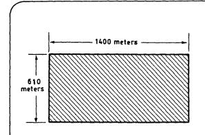
FIG. 4 \_ APROXIMATE GROUND SIZE COVERAGE PER SCREEN, FOR NON CORRECTED CCT. (h=1 km)
