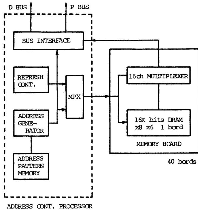
Fig. 2 The Block Diagram of Memory I/O System.
