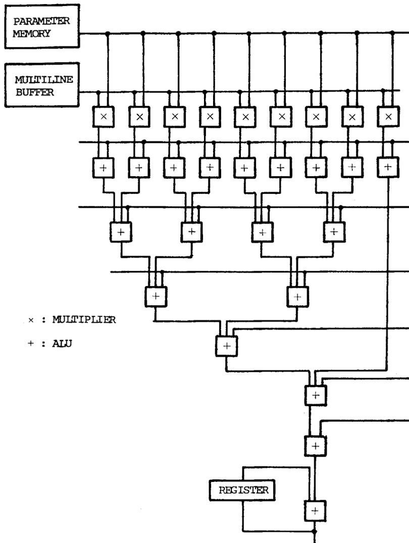
Fig. 3 A Standard Configuration of ALU Array Processor.
